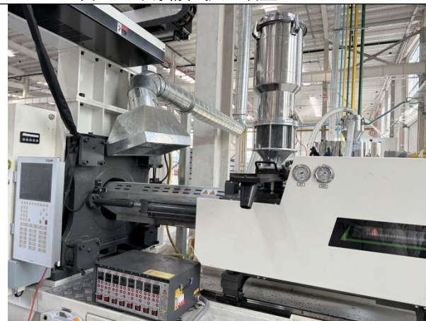
图3-3 注塑机集气罩
